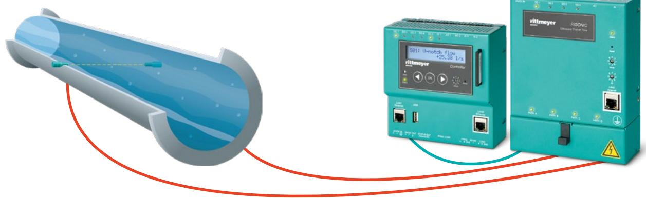
The flow measurement is based on the acoustic discharge measurement (ADM) method. Sensor A and B alternately send and receive an ultrasonic waveform. The measured transit time difference of the two waveforms is directly proportional to the mean path velocity. From the mean path velocity in conjunction with the pipe geometry the flow can be determined.
